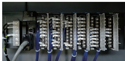
Optimal operational logics with varying required air guaranties : PLC based controller
